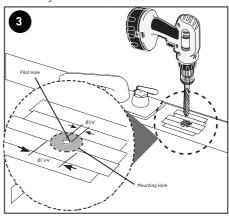
4. Drill hole for filter faucet installation
